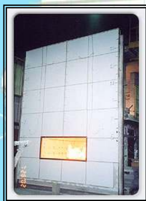
6. Start of the UBC 26-9 ISMA Test
