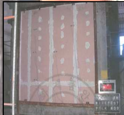
Unexposed face of the specimen before Fire Test
