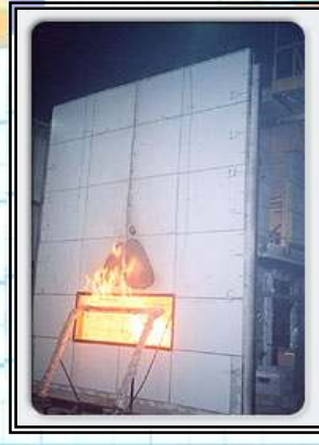
8. 15 min. Into the UBC 26-9 ISMA Test
