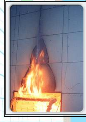
9. 25 min. Into the UBC 26-9 ISMA Test
